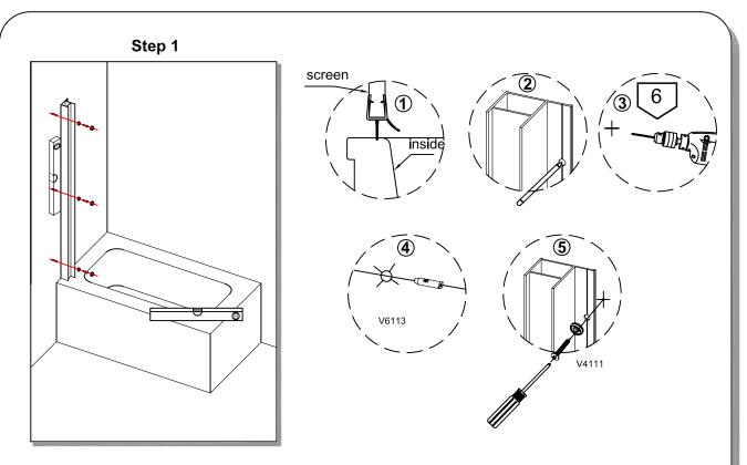
**Step 1.**Position the wall profile so the seal on the moving panel sits over the inside edge of the bath screen. Fix wall profile using screw V4111.
